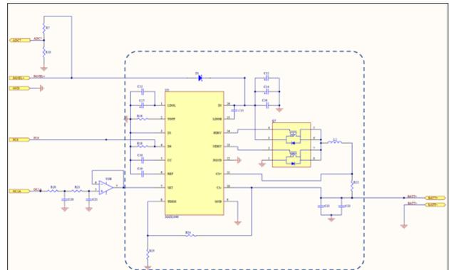
Fig. 3. Charger circuit for testing and tuning the MPPT algorithm.
