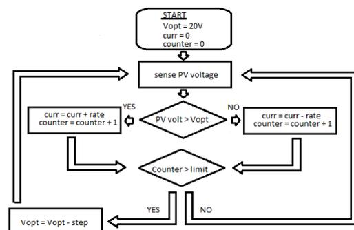
Fig. 1. Flow chart of the proposed MPPT algorithm.
