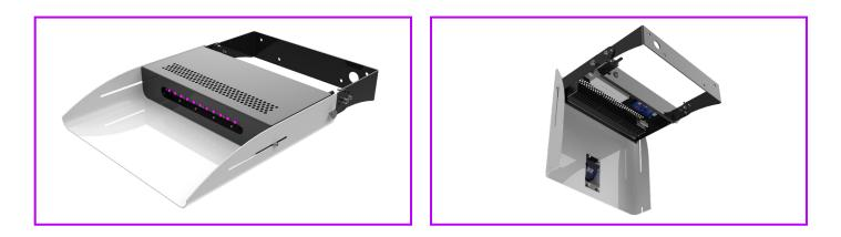
This smart device reduces the viral load in room air by using 265 nm UV-C LED technology. Thanks to the integrated motion sensor, it adjusts the disinfection of the air to the movement detected in the rooms in an efficient way, without exposing the occupants to irradiation.
